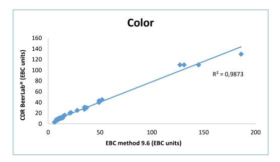
Figure 3 Correlation between color units measured with CDR BeerLab<sup>®</sup> and EBC method 9.6.
