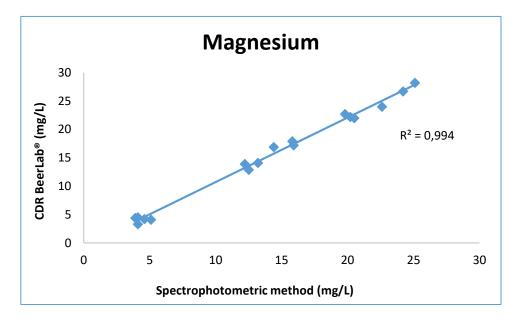
Figure 11 Correlation between magnesium content in water with CDR BeerLab<sup>®</sup> and spectrophotometric method.
