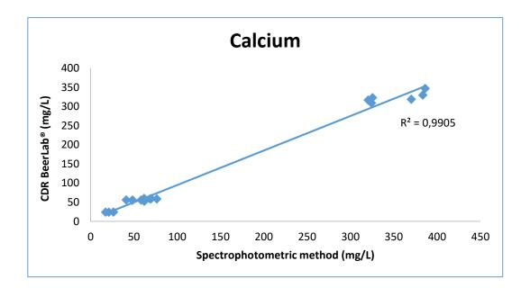
Figure 10 Correlation between calcium content in waters with CDR BeerLab<sup>®</sup> and spectrophotometric method.
