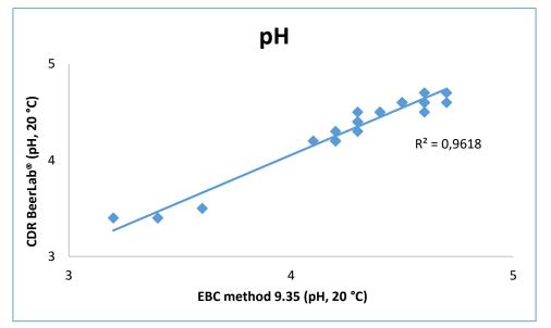
Figure 2 Correlation between pH values measured at 20 °C with CDR BeerLab<sup>®</sup> and EBC method 9.35.
