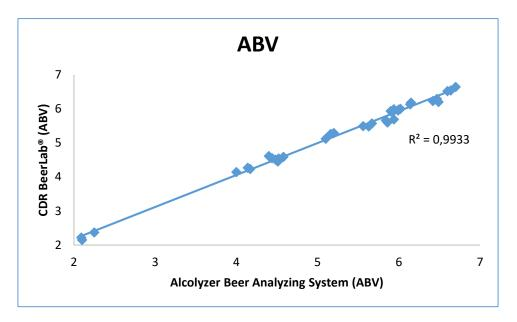
Figure 1 Correlation between ABV values measured with CDR BeerLab<sup>®</sup> and Alcolyzer Beer Analyzing System.
