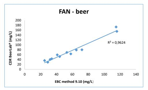
Figure 5 Correlation between FAN content in worts measured with CDR BeerLab<sup>®</sup> and EBC method 9.10.
