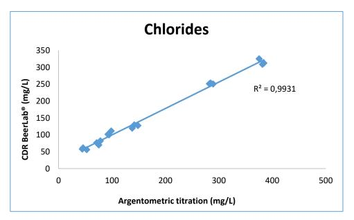
Figure 13 Correlation between chlorides content in water with CDR BeerLab<sup>®</sup>r and argentometric titration.
