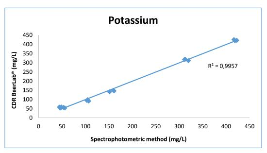
Figure 12 Correlation between potassium content in water with CDR BeerLab<sup>®</sup> and spectrophotometric method.
