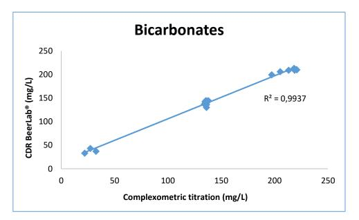
Figure 16 Correlation between bicarbonates content in water with CDR BeerLab<sup>®</sup> and complexometric titration.
