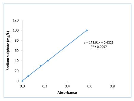
Figure 14 Calibration curve for the turbidimetric analysis of sulphates.
