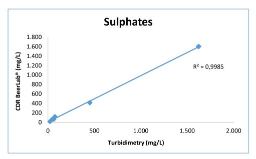
Figure 15 Correlation between sulphates content in water with CDR BeerLab<sup>®</sup> and turbidimetry.
